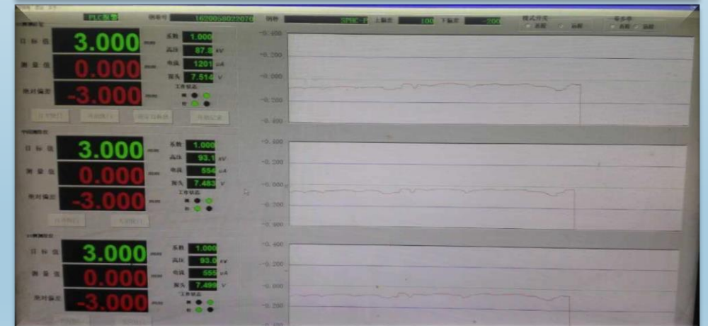
Online edge drop gauge thickness measurement system
